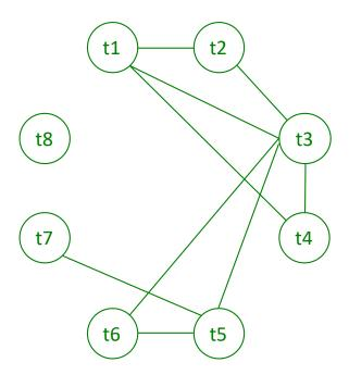
(b) (6 points) Give an assignment of groups of temporary variables to registers that uses the minimum number of registers possible based on the information in the interference graph. Use R1, R2, R3, ... for the register names.
