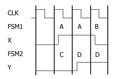
machines advance in lock step initial inputs/outputs: X = 0, Y = 0
