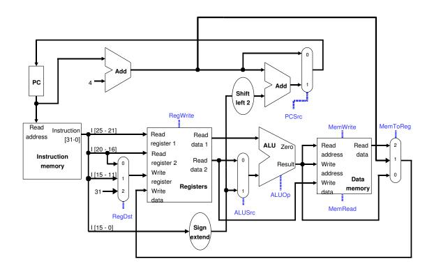
Given the single-cycle datapath above (control signals are marked with dashed lines), fill in the blanks in the table below. You must either give the control signals (0, 1, X) for a particular MIPS instruction, or give the MIPS instruction that uses the specified control signals.
