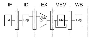
The or has a data dependence on the add, and the addi on the lw. Since we have no forwarding, we need to allow 2 cycles between the dependent instructions, so that the producer can reach WB when the consumer is in ID.
