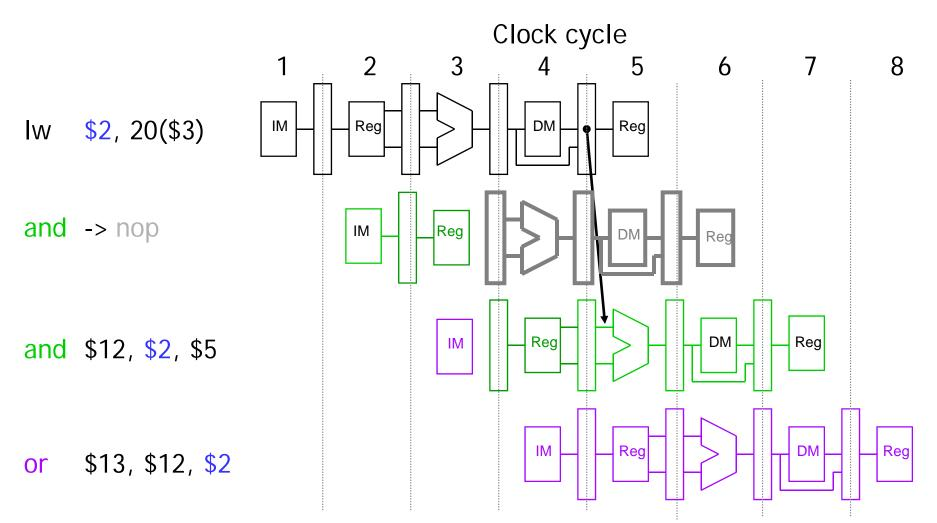
The effect of a load stall is to insert an empty or nop instruction into the pipeline Detecting stall is much like detecting data hazards.
