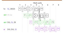
• The effect of a load stall is to insert an empty or nop instruction into the
