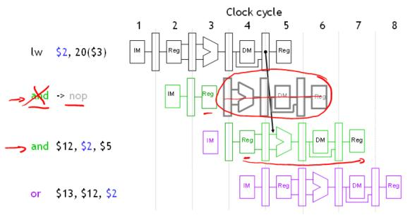
The effect of a load stall is to insert an empty or nop instruction into the pipeline
