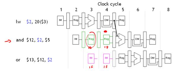
■ Those units aren't used in those cycles because of the stall, so we can set the EX, MEM and WB control signals to all 0s.
