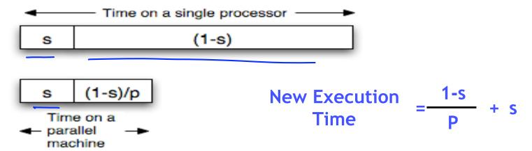
• For example, consider a program that, when executing on one processor, spend 10% of its time in a non-parallelizable region. How much faster will this program run on a 3-processor system?
