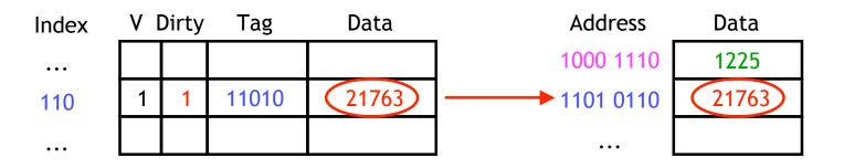
• Only then can the cache block be replaced with data from address 142.
