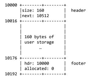
A common class of bugs in the implementation of getmem/freemem is for the header or footer to become corrupted. To check for such bugs, your job is to write a check\_list function for the freelist. This function should check the following properties for every block in the freelist, using assert:
