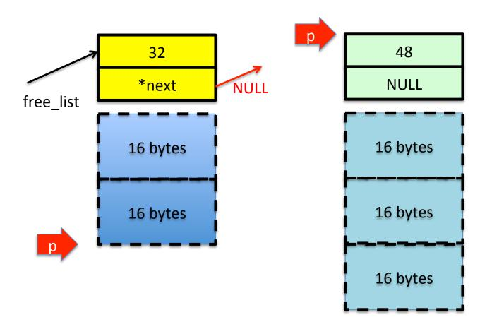
When freemem returns a block of storage to the pool, if the block is physically located in memory adjacent to one or more other free blocks, then the free blocks involved should be combined into a single larger block, rather than adding the small blocks to the free list individually.
