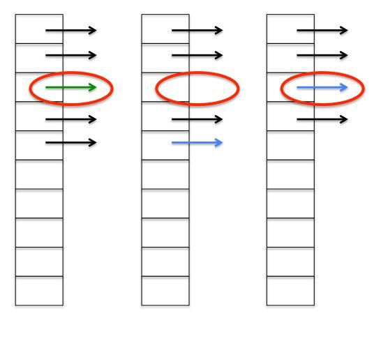
Holds pointers returned by getmem function. Maximum size of n\_trials. Fill from position 0 onwards (entire array may not ever be full). The freemem function randomly chooses one element from filled part of array to return to the free\_list. Fill the gap in O(1) time by moving the bottom element into the gap and shortening the length of the filled part of the array.
