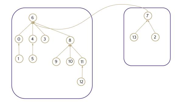
Given the following disjoint-set what would be the result of the following calls on union if we add the "union-by-weight" optimization. Draw the forest at each stage with corresponding ranks for each tree.
