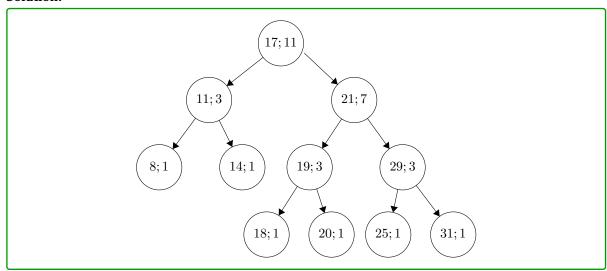
ii. Given a modified AVL tree, like the one above, describe a procedure that will return the median element stored in the tree. Note that in the modified tree, you can access the number of elements lying below a node in addition to the number stored in that node. Can you use this extra information to find the median more quickly?
