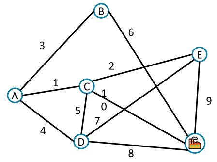
She knows how much it would cost to lay electric wires between any pair of locations, and wants the cheapest way to make sure electricity from the plant to every city.
