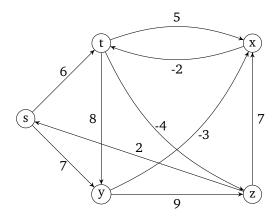
Suppose we run Dijkstra's algorithm on this graph starting with vertex s. (Note: we will very likely get meaningless results due to the negative edges, but this is still a good way to practice running the algorithm.) What are the final costs of each vertex and the shortest paths from s to each vertex?
