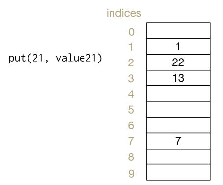
Note: For simplicity, the table shows only keys, but in each slot both, key and value, are stored.
