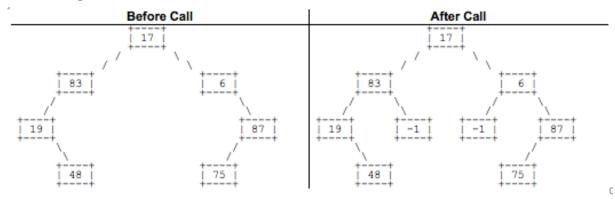
In this case, the request was to fill in nodes as necessary to ensure that the first 3 levels are complete. There were two nodes missing at level 3. Notice that level 4 of this tree is not complete because the call requested that nodes be filled in to level 3 only.
