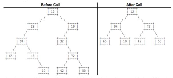
The nodes that stored the values 28, 19, 32, and -8 have been eliminated because each had one child. When a node is removed, it is replaced by its child. This can lead to multiple replacements because the child might itself be replaced (as in the case of 19 which is replaced by 32 which is replaced by 72).
