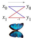
A data-flow diagram connecting the inputs  $x$  (left) to the outputs  $y$  that depend on them (right) for a "butterfly" step of a radix-2 Cooley-Tukey FFT. This diagram resembles a butterfly.
