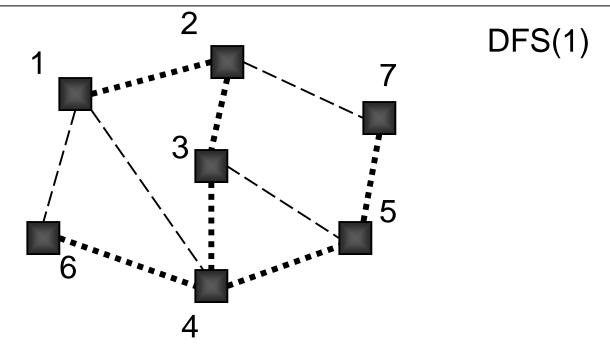
All nodes are marked so graph is connected; red links define a spanning tree
