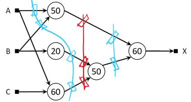
The key is to break up the critical path along the bottom; the NOT gate must be in the  $1^{st}$  stage while the upper AND gate can be placed in the  $1^{st}$  or  $2^{nd}$  stage as long as it isn't part of the new critical path.
