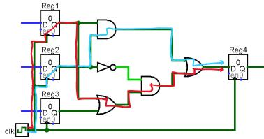
**Longest data path** and **shortest data path** are shown on the circuit diagram above (note that the clock network delays are ordered  $t_{clk1} > t_{clk2} > t_{clk3}$ ). Both paths have Reg4 as their destination register for the clock paths.
