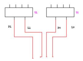
And feed these four outputs to some logic which using them solves for the **P** and **Y**. However in the cases in which the pattern in between the two four inputs would not be detected. (for e.g. **I=0001 0100 or I= 1110 1000**). Therefore three such blocks are required each with Inputs  $I_7I_6I_5I_4$ ,  $I_5I_4I_3I_2$  and  $I_3I_2I_1I_0$  respectively).
