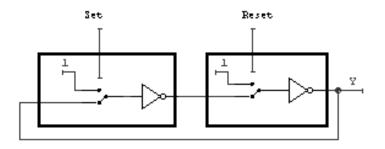
□ Now, take a look at the black boxes above. Each has two inputs. When the first input is 1, the output should go to 0, whereas when the first input is 0, then the output should be the negation of the second input. What is that?
