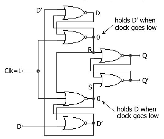
negative edge-triggered D flip-flop (D-FF)
