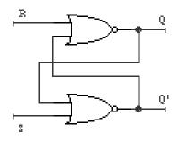
☐ This is called an R-S latch. We can build a table that shows how this circuit behaves:
