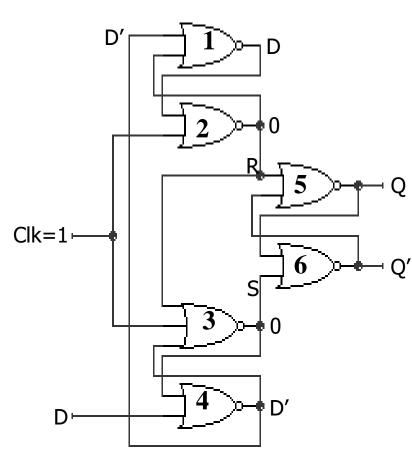
Setup time: Time data must be stable before negedge of clock to ensure proper latching. Where does D wait for falling edge of clock? at G2 and G3.  $T_{su} = 2$
