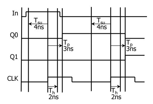
timing constraints guarantee proper operation of cascaded components
