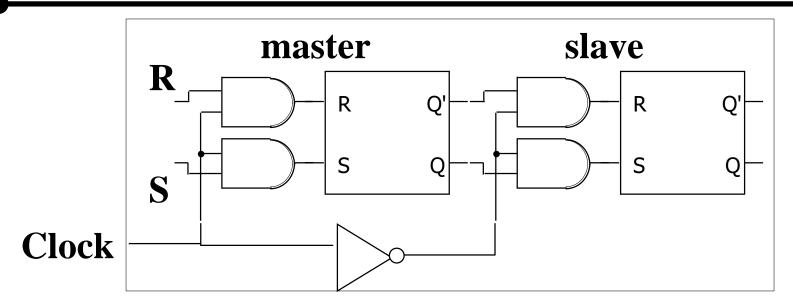
Changes on inputs can't propagate to outputs until next clock cycle begins.
