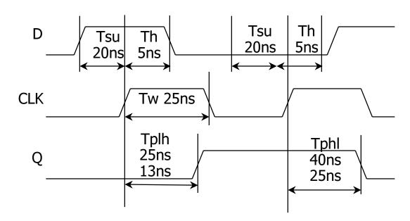
all measurements are made from the clocking event that is, the rising edge of the clock
