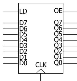
OE asserted causes FF state to be connected to output pins; otherwise they are left unconnected (high impedance)
