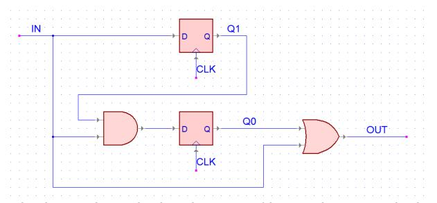
Complete the timing diagram that shows the execution of the circuit above. Assume that the gates and registers have a delay of 1ns. The vertical dotted lines break the time line into 1ns sections. (Thus the clock period is 8ns.) You do not have to think about setup and hold times.
