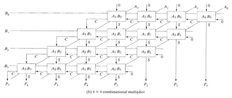
Figure 5.26  $4 \times 4$  combinational multiplier.
