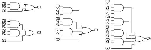
Logic complexity increases with adder size
