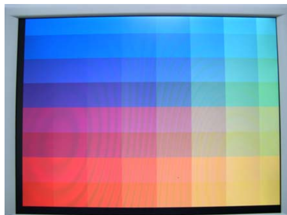
Figure 2.3. The default VGA output pattern when SW0 is set to DOWN position.
