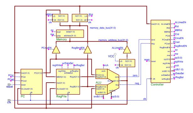
Below is the architecture diagram for the processor of Assignment #9 and #10.
