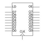
OE asserted causes FF state to be connected to output pins; otherwise they are left unconnected (high impedance)
