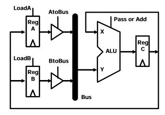
(a) Show the register-transfer operations needed to implement an instruction that swaps the contents of the A and B registers (SWAP A, B). Use as many cycles as you need to implement the instruction (up to 4) and note the value of each control signal in each cycle. Assume the instruction is already in the instruction register so there is no need to worry about fetching the instruction or incrementing a program counter.
