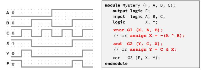
(B) A testbench for the Mystery module (with inputs A, B, C) is shown below. Which input combinations are NOT currently being tested? You may not need all of the blanks. [3 pts]
