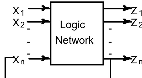
The presence of feedback introduces the notion of “state.”
