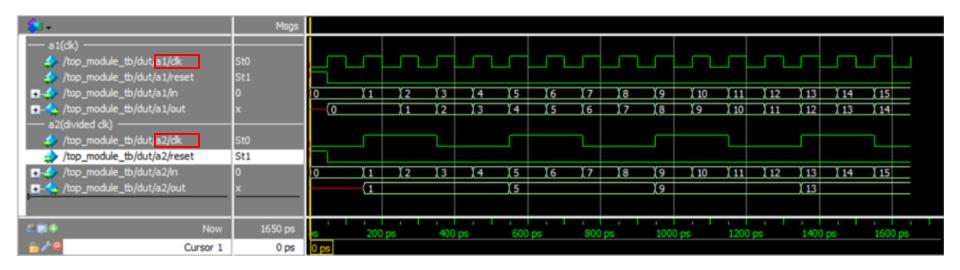
The clocks in module a1 and a2 have different clock frequency. Module a2 has a slower clock than a1 does, causing desynchronization issue.
