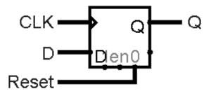
Option 2: asynchronous reset
