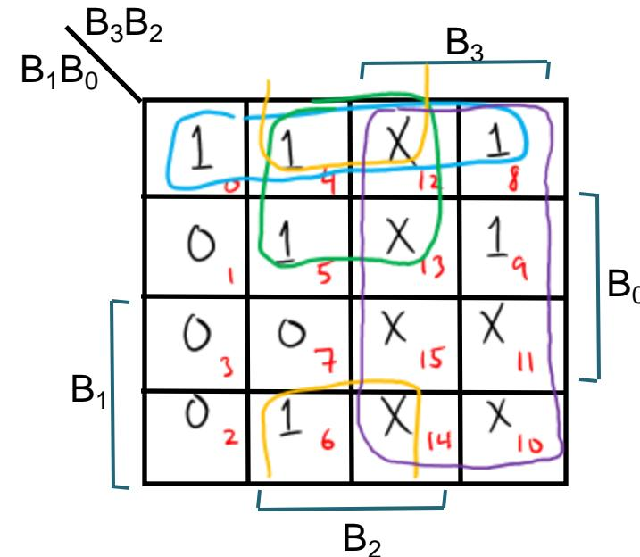
$$L5 = \bar{B}_3 \bar{B}_0 + B_2 \bar{B}_1 + B_2 \bar{B}_0 + B_3$$
