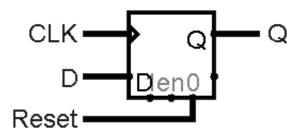
Option 2: asynchronous reset
