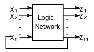
Network implemented from logic gates. The presence of feedback distinguishes between sequential and combinational networks.
