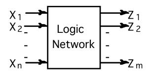
No feedback among inputs and outputs. Outputs are a function of the inputs only.
