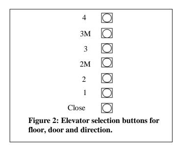
The system, as it currently stands, will go to the floor specified based on the floors that are pressed and by the direction the elevator is already going. You do not have to worry about calling the elevator. The department has decided that our Undergraduate Advisor will be able to see many more students by running the elevator. What you do have to deal with is a passenger entering the elevator should be able to press the button for the floor he or she wishes to go to.
