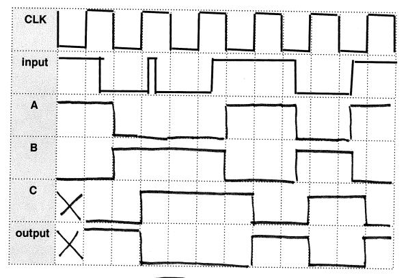
Part 2 (5 points): Is this a positive edge triggered flip flop or negative edge triggered flip flop?
