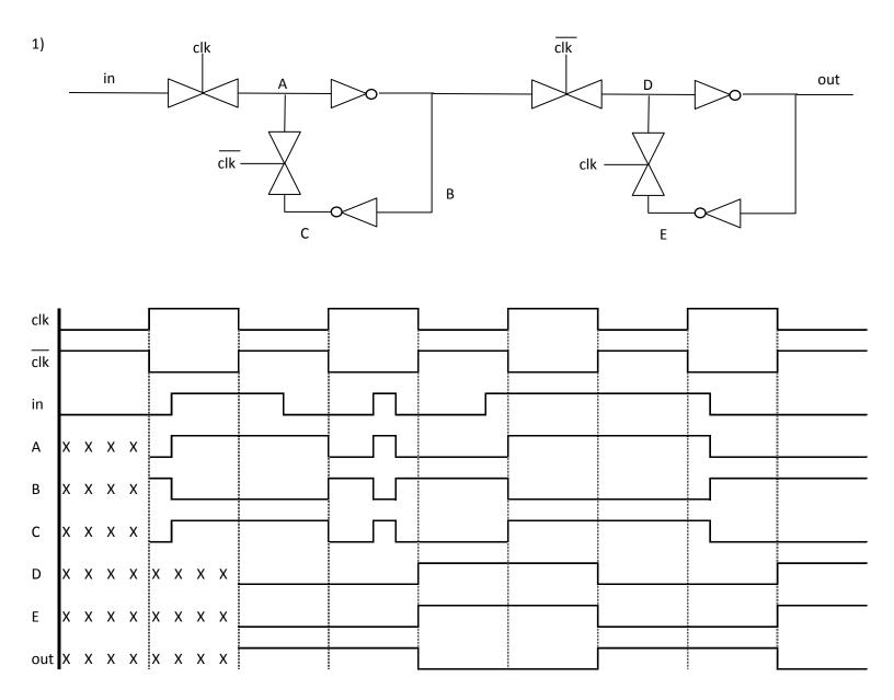
Fill in the chart above with the appropriate signals. Mark X's in regions where the signal state is not known.
