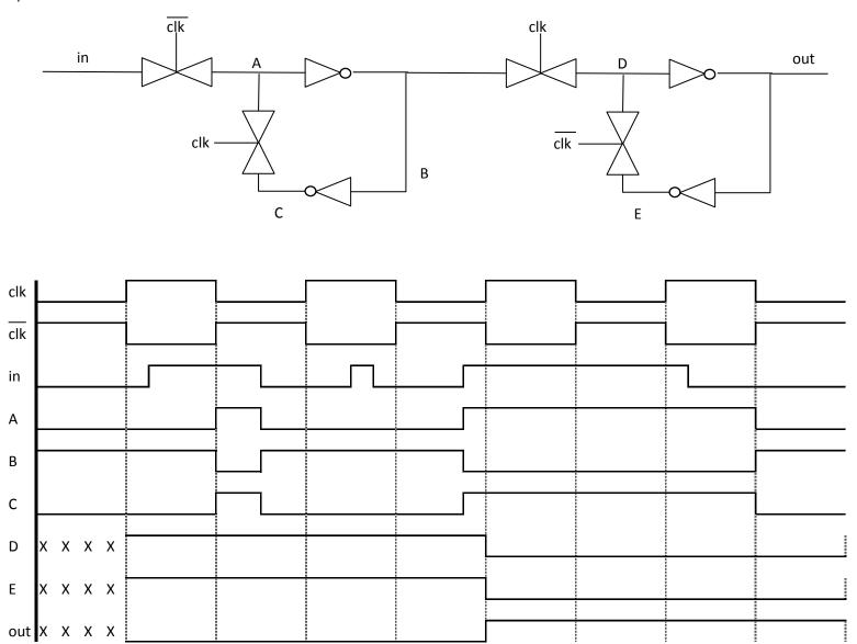
Fill in the chart above with the appropriate signals. Mark X's in regions where the signal state is not known.
