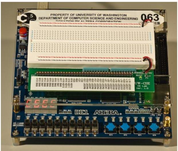
The red line marks where VDD runs across the board, and the black line marks were GND runs across the board. The holes on the board are interconnected as the blue line shows, up-and-down for each 5-hole segment.
