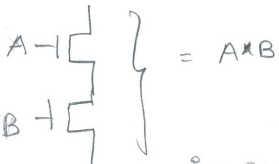
Two nmos connected in series (cascade) implements "and" function
