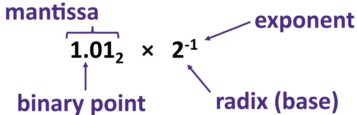
The diagram illustrates the components of the binary scientific notation  $1.01_2 \times 2^{-1}$ . The mantissa is  $1.01_2$ , with a bracket above it labeled "mantissa". The binary point is the dot in  $1.01_2$ , with an arrow pointing to it labeled "binary point". The exponent is  $-1$ , with an arrow pointing to it labeled "exponent". The radix (base) is  $2$ , with an arrow pointing to it labeled "radix (base)".
