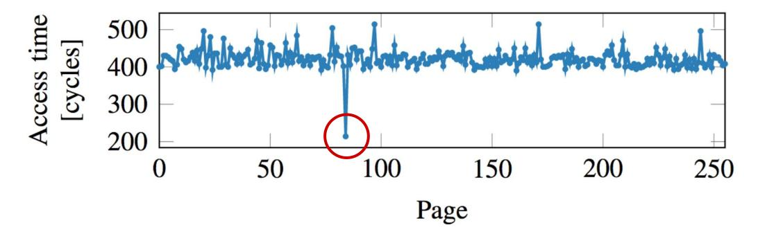
Access probe\_array[data \* 4096], timing the access for a cache hit. If hit detected, the value of data is the byte read from the kernel address!!!
