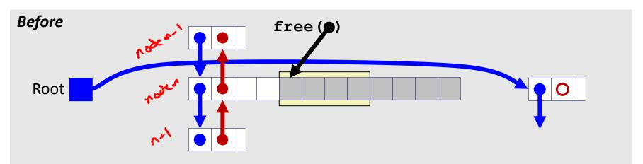
Splice <u>preceding</u> block out of list, coalesce both memory blocks, and insert the new block at the root of the list
