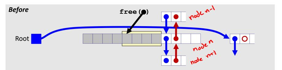
Splice *following* block out of list, coalesce both memory blocks, \* and insert the new block at the root of the list
