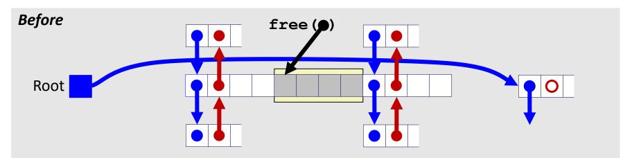
Splice <u>preceding</u> and <u>following</u> blocks out of list, coalesce all 3 memory blocks, and insert the new block at the root of the list
