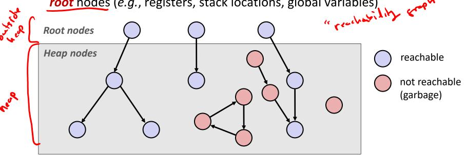
A node (block) is *reachable* if there is a path from any root to that node Non-reachable nodes are *garbage* (cannot be needed by the application)
