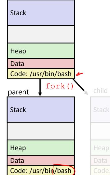
Very high-level diagram of what happens when you run the command "ls" in a Linux shell: This is the loading part of CALL!
