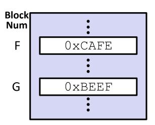
Step: Write 0xFEED to cache only (and set the dirty bit)
