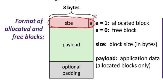
e.g. with 8-byte alignment, possible values for size:
