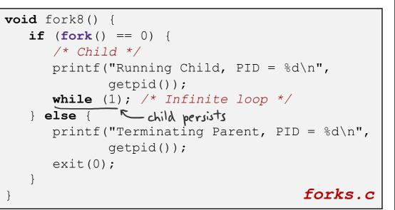
linux> ./forks 8 Terminating Parent, PID = 6675 Running Child, PID = 6676 linux> ps PID TTY TIME CMD 00:00:00 tcsh 6585 ttyp9 00:00:06 forks 6676 ttyp9 6677 ttyp9 00:00:00 ps *linux>* kill 6676 *linux>* ps PID TTY TIME CMD 6585 ttyp9 00:00:00 tcsh 6678 ttyp9 00:00:00 ps
