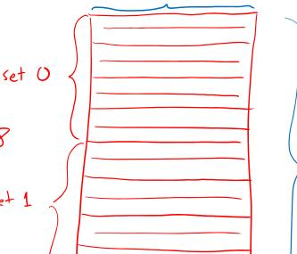
\* If addresses are 16 bits wide, how wide is the Tag field?  $k = log_2(K) = 7 bits$ ,  $s = log_2(5) = 1 bit$ , t = m - s - k = 8 bits
