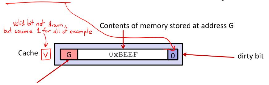
tag (there is only one set in this tiny cache, so the tag is the entire block address!)
