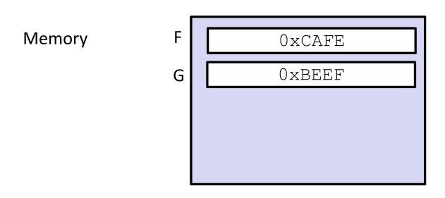
In this example we are sort of ignoring block offsets. Here a block holds 2 bytes (16 bits, 4 hex digits).
